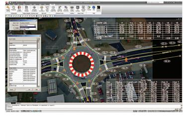
>> The roundabout design is instantly updated when edits are made to different elements such as approach lanes and exit radius.
