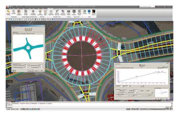
>> Easy to use grading model allows engineers to define profiles, spot elevations, and cross slopes.
