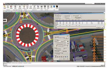
Set instant visual feedback for fastest path assessment. Review roundabout geometries based on the fastest path of a vehicle moving through the design.
