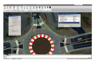
>> Generate various types of sight lines in the drawing. Existing sight lines can also be edited and removed. Sight line analysis is important for determining safety constraints in a roundabout.
