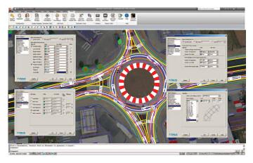
>> Select and view different roundabout iterations from your saved files for project decision making and client review. Each roundabout design can have its own design symbol and independent set of iterations.
